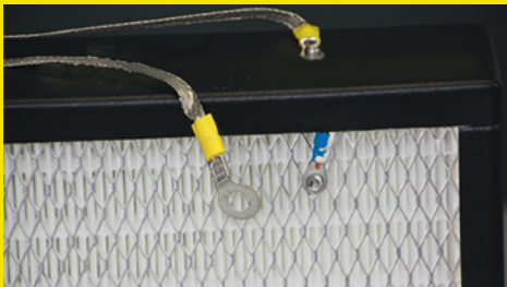
EMW® ATEX filter boxes and panel filters are supplied with integrated earthing lugs. EMW® compact filters have pre-formed mounting recesses on the inlet and outlet sides of the filter frame. Their earthing lug, supplied with the filters, can be conveniently mounted on either side as desired.
